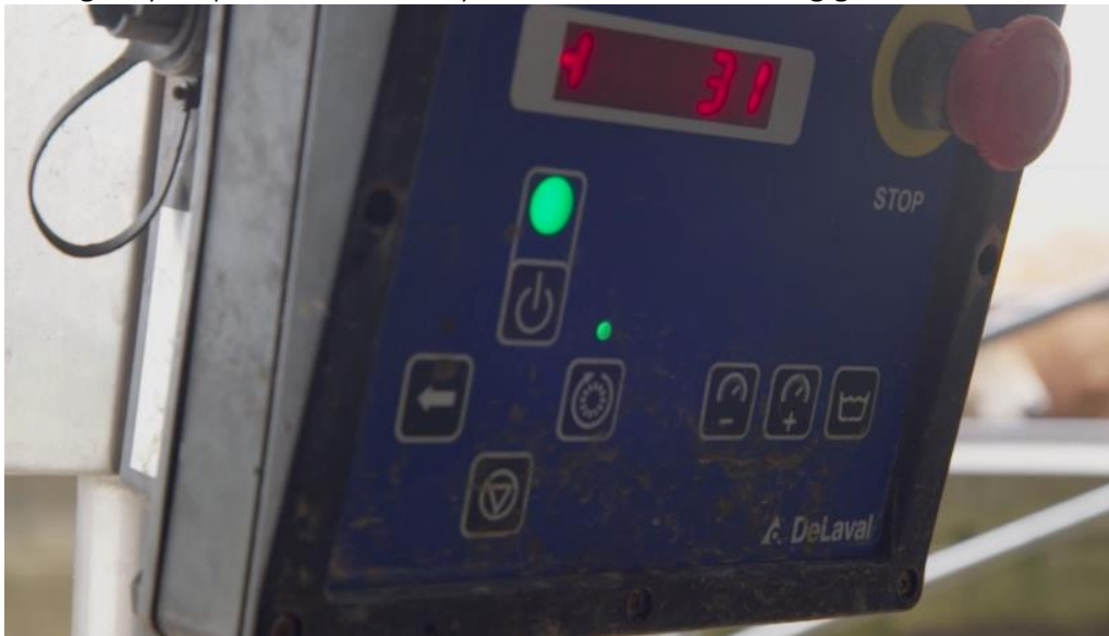
Fig. 1: The control panel allows you to control the basic functions of the rotary platform, and has an emergency stop
