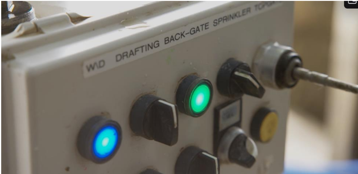
Fig. 2: The control panel also lets you control the backing gate
